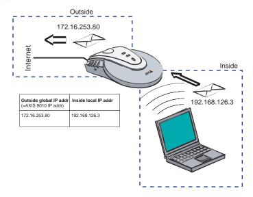
IP Masquerading uses almost the same method for IP translation as NAT (Network Address Translation), except that masquerading also uses the port number in the translation.
