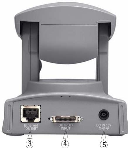
③ **Network Connector** - The AXIS 213 connects to the network via a standard RJ45 connector. Supporting NWAY, the AXIS 213 detects the speed of the local network segment (10BaseT/100BaseTX Ethernet).
