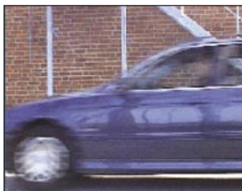
Interlaced, 20 ms difference between odd and even lines
