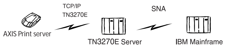
Typical AXIS 5570e/AXIS 5670e TCP/IP TN3270E Network Configuration
