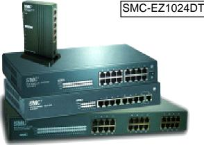
This EZ 10/100 series offers 5-, 8-, 16-, and 24-port 10/100 Mbps standalone, unmanaged switches. Designed specifically for home and small office applications, these switches feature auto-negotiation, uplink ports for easy network expansion, and provide bandwidth capability on each port. With fully auto-negotiating 10/100 ports, the speed and duplex modes of attached devices are instantly detected, allowing the switches to auto-configure for optimal performance.
