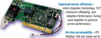
High performance and flexibility -10/100 and full-duplex auto-negotiation, 802.1Q VLANs. 802.3x flow control.
